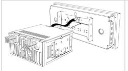
Plug the ribbon cable from the Radio Motor into the Radio Face.
