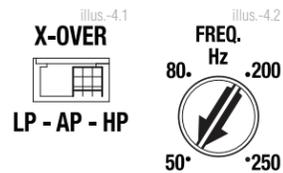
Placing the crossover switch in the HP position sets the amplifier to the High Pass mode, enabling frequencies above the cut-off point to pass, adjustable between 50-250Hz.
