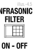
NOTE: We recommend using the infrasonic filter when using vented enclosures with this amplifier.
