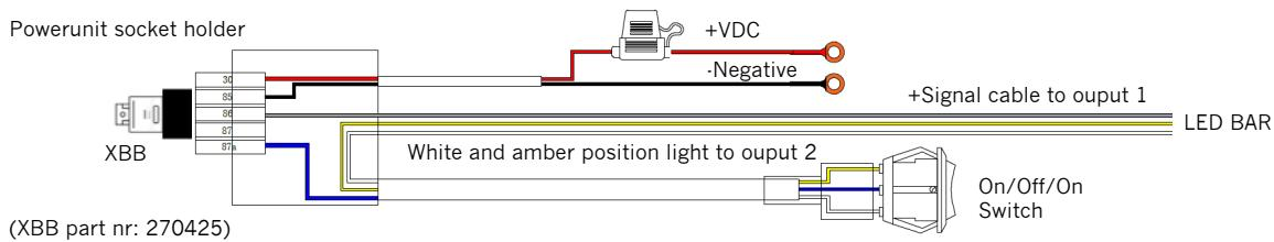
**Note:** This wiring harness is designed for connecting an XBB Power Unit. The Power Unit or relay are not included in the package. The On/Off/On switch is for two-position lights; if this feature is not needed, you do not need to connect any wires to the assigned wire in the harness, easy to use for lights with a built-in relay. For those lights without a built-in relay and power above 15A, an extra relay cable harness is required.
