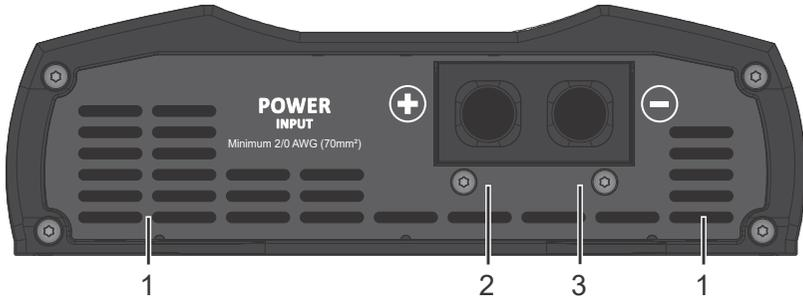
**1 - FANS:** This amplifier has two internal ventilation fans, and cannot be blocked. For perfect functioning, the amplifier must be installed in a cool and aired place. It is recommended not to embed it, so that the air circulates throughout the inside of the product extension, thereby preventing the thermal protection from acting.
