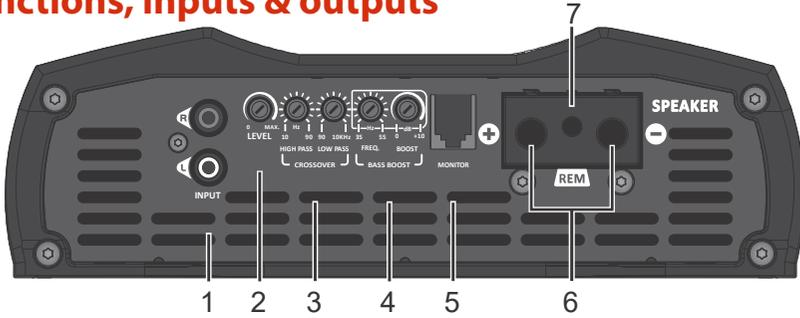
**1 - INPUT (R and L):** Inputs of signals to be amplified. Connect these signals to RCA outputs of Head Unit, using good quality shielded cables to avoid noise influence.
